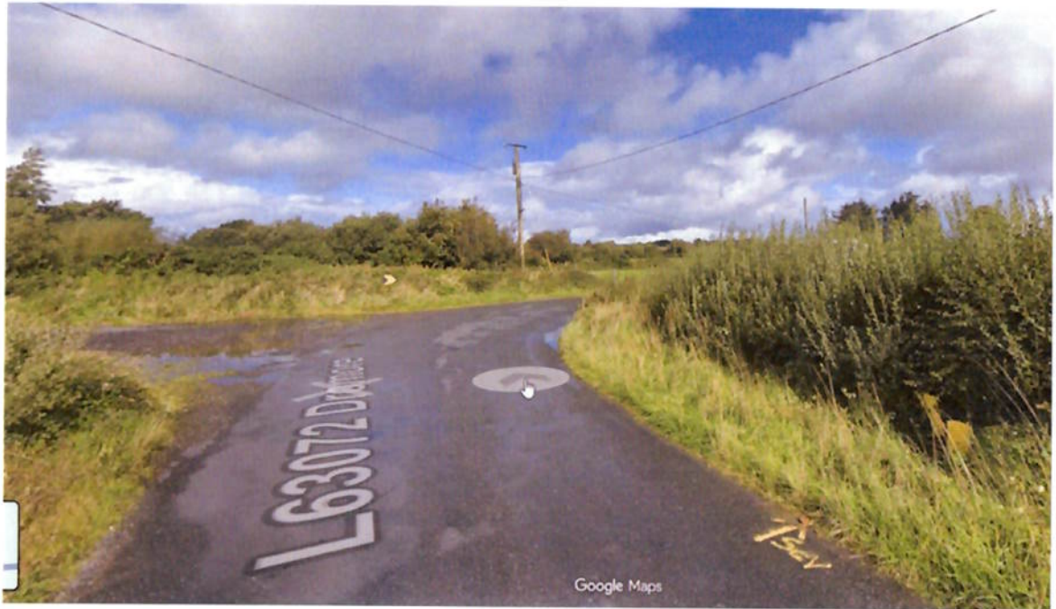
Figure G2. Street View imagery at the Location 17 bend. The overhead electricity line can be seen running between the roadside poles. The upper-bend electricity pole forms part of the connection serving the observer's dwelling, with the line continuing towards the pole beside the property. The right-hand roadside pole is identified by the observer as telecommunications infrastructure.
